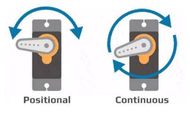
As name suggests, continuous servos keep on rotating, and the positional servos move to a specific position. For example, a positional servo is used to steer the wheels on a car robot or to turn the camera to a specific direction.
