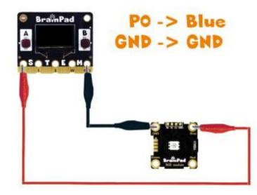
We now want to control all three primary colors. Connect 4 alligator clip wires as shown in this diagram.
