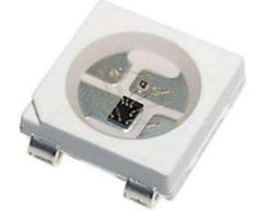
Those smart LEDs are chained and, therefore, they all can be controlled from a single pin on the controller. The "controller" in this case is BrainPad Pulse. The smart LED in the BrainClip kit is the LED Ring module.
