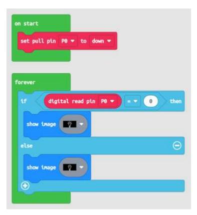
Have you noticed how we check for a "0" state on the pin to turn the light on? This is because we are using a block to pull the PO high/up. Measuring the pin on the button module will result in "1", which is high/up. Pressing the button will make a connection between the pin and GND, making the pin "0". This maybe seems backwards to you, but this is normal practice when connecting a button.
