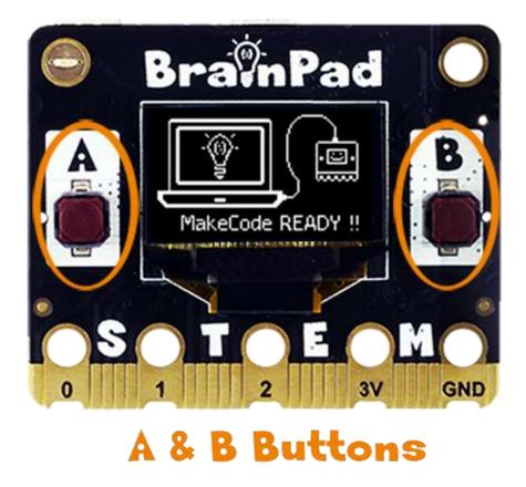
If you hold A and B buttons for 5 seconds and screen does not show the "**MakeCode READY!!**" image, then your board is loaded/prepped to do other languages, like Python or .NET C#. Fear not, you can change it back to MakeCode as shown on the MakeCode Setup lesson <a href="https://www.brainpad.com/lessons/makecode-setup/">https://www.brainpad.com/lessons/makecode-setup/</a>.
