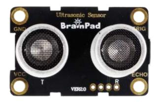
Sending a pulse starts with TRIG pin, the trigger. The response with the distance comes back on the ECHO pin. We will use TRIG on P0 and ECHO on pin P1.
