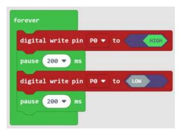
Load the program onto BrainPad Pulse and the RGB module should blink Red, awesome! Move the alligator clip from the Red pad to the Blue pad on the RGB module and the LED will now blink Blue.
