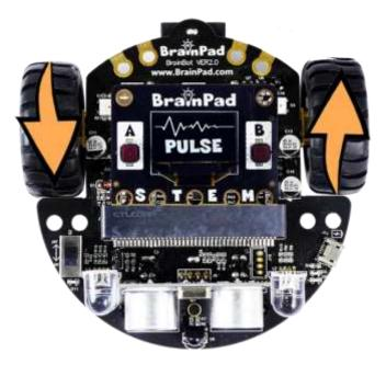
The other option is to stop one of the wheels and move the other. This will make the robot turn in a larger radius.
