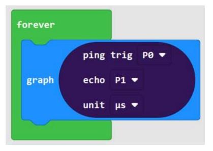
Keep in mind the sensor uses the sound reflection to measure distance. It will, therefore, work best with solid and flat surfaces.
