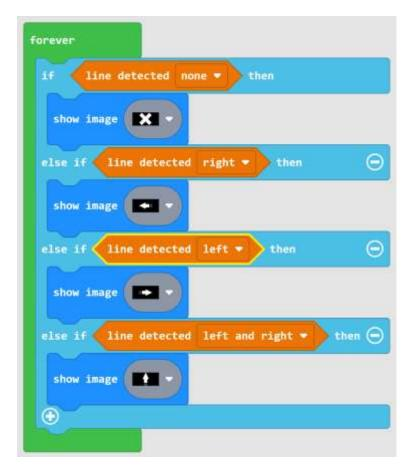
The black line on the sheet fits right in between the two sensors, resulting in detection to being none. We are showing the X image to indicate that no lone is being detected. Place the robot on the sheet, over the line. Rotate the robot slightly right and left and observe the screen.
