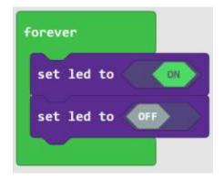
This forever loop will now turn the LED on and off forever, blinking the LED. But the LED on the simulator is not blinking, is it? Well, I promise you it is blinking, but you are just not seeing it. It may flicker but will not blink properly. This is because the loop is running just too fast for our eyes to see it. This will be true if we were to run this loop on the circuit. This is an example of where debugging comes in handy.
