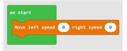
The speed can be set to a positive number, for going forward, and a negative number for going backwards.
