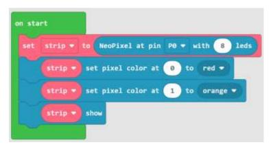
Note how the show block is required. Set pixel color block only tells the driver what we want, but it does not send the signal to the LEDs yet. Only when the show block is used the signal will be sent.
