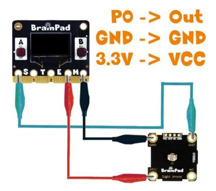
We can use the light level to detect it is nighttime and, therefore, turn the porch light on, for example. This example, however, will graph the light level.
