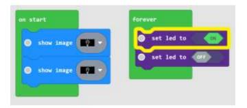
The LED on the simulator will work just fine, matching the blocks. Have we just found the bug? The problem in this case is simply speed. The LED is blinking, but it is too fast for our eyes to see.
