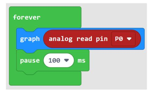
Change the light level around the sensor and observe the screen.
