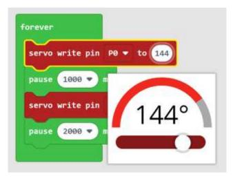
A loop can send the servo back and forth indefinitely.
