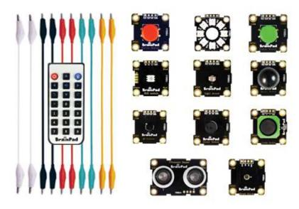
The modules can be connected to BrainPad Pulse using those clip wires.
