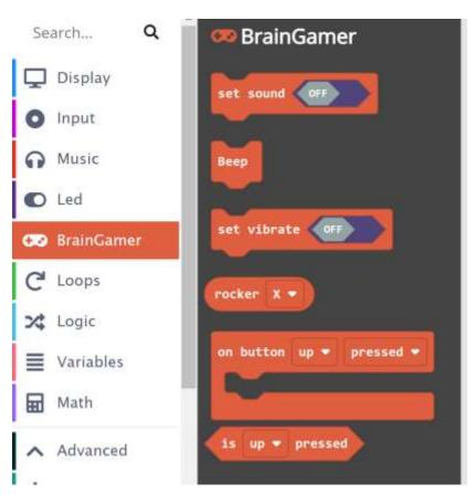
The BrainGamer buttons can be used similarly to how we used the A and B buttons before. Note that while the BrainPad circuit labels the buttons as A, B, X, and Y, the extension uses up, down, left, and right to eliminate any confusion with the A and B buttons on BrainPad Pulse.
