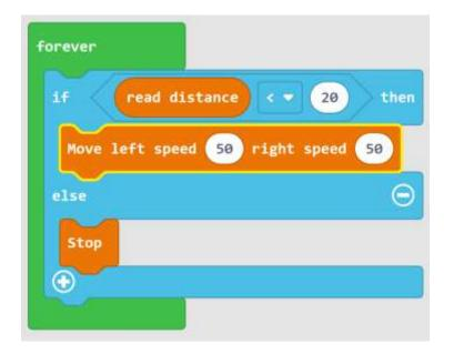
The robot can also use distance measurement to avoid obstacles. The used algorithm is very simple. If the robot detects a distance less than 20cm, it will turn for 200ms and then try to go forward again.
