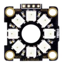
The RGB pad is where the signal comes in to the 8 smart RGB LEDs.
