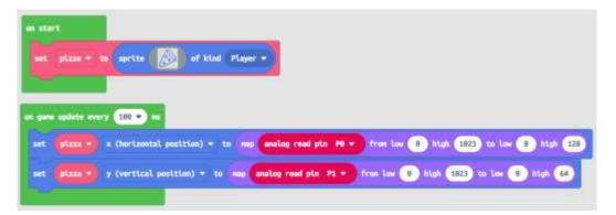
You will notice that the sprite moves left and right properly, but it is inverted in the Y (up and down) direction. This is because the display starts with zero location at the very top left, where the rocker starts with zero at the bottom.
