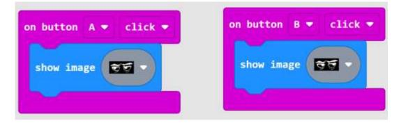
At first, nothing will show on the screen as we have not added anything to on start block. Now try the A and B buttons. Pressing each one of the buttons will show its image on the screen.
