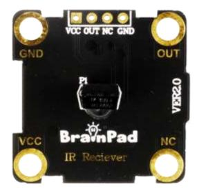
The OUT pin is the signal that needs to be decoded.
