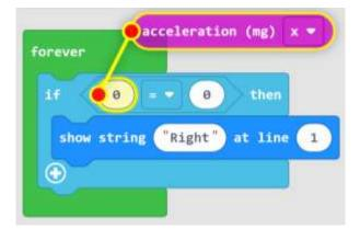
MakeCode will help by showing a line to an appropriate spot for the block. The acceleration outputs a value that is maxed at 1023 in one direction and -1023 on the other direction. The output will be zero right in the middle. Let's compare the value to be more than 500.
