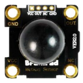
We will use this sensor to create an alarm. The OUT pad goes to P0, with power and ground connecting as usual.
