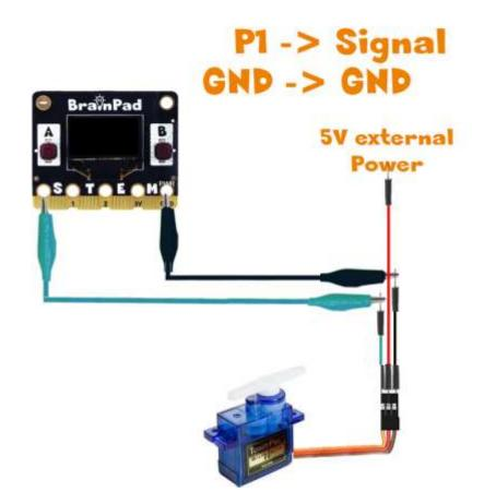
The "servo write" block is found under pins, under advanced. The block accepts 0 to 180 degrees, which is the angle of where the servo will be pointing.
