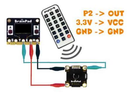
To decode IR signals, we need the infrared extension.
