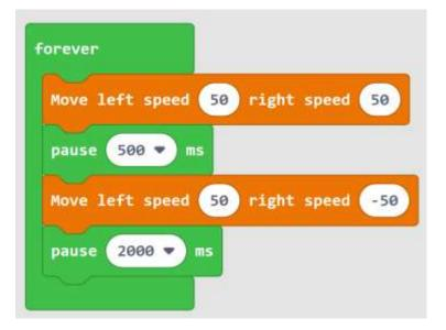
Can you change the blocks so the robot is moving as it is going around a square? The blocks are the same, you just need to change the timing and the speeds.
