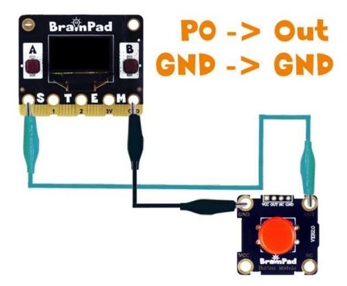
The code will use the button to control the lightbulb on the screen.
