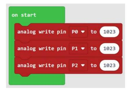
The analog value allowed for analog write is 10bit in resolution, which is where the 1023 comes from. Two to the power of 10 is 1024, allowing for value 0 to 1023. If we are using a color picker tool, we need to scale/map the values from 255 max to 1023 max.
