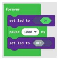
The LED is starting to flicker on the simulator, but it is still not blinking. Let's analyze the forever loop. An LED is turned on, a pause stops the program for 1sec, so the LED will be lit for a whole second. Then a block turns the LED off. But immediately after that, the forever loop will rerun the LED on block. The LED was, in fact, off but for a very short time. Let us add a second pause.
