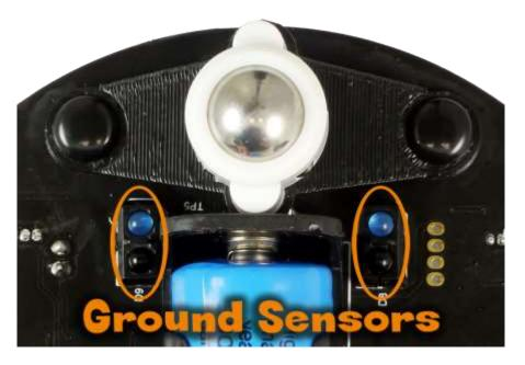
The ground sensors use the ground to reflect an infrared beam back to a light sensor located next to them. If you look closely at them, you'll see a separator between both. This is so it only gets the value from the reflection off the ground and not spill over from the beam itself. The infrared light sensor may look black to our eyes, but it is designed to filter out all other light except the infrared.
