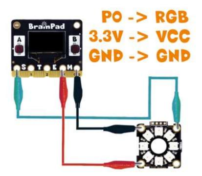
The special signal that needs to be generated to control those smart LEDs is found in the neopixel extension. Go to Advanced options under the block menu and click on Extensions. Now add the neopixel extension.
